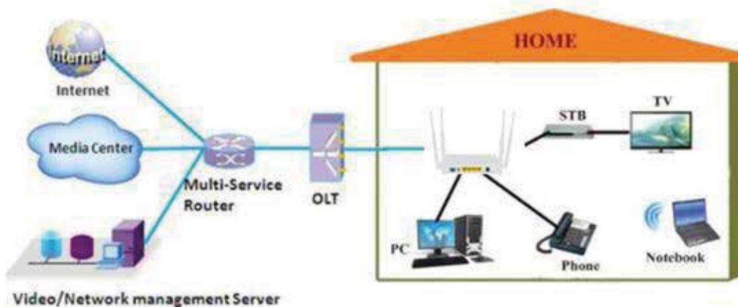
Picture 1-1 FD-HG8421A products Network diagram
